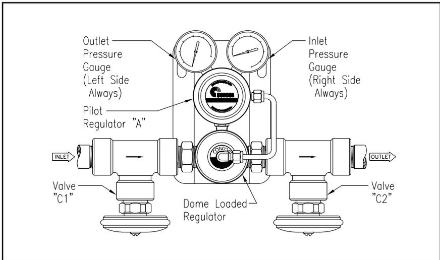
Figure 1. 623 Series Dome Load Regulator and Valves,
