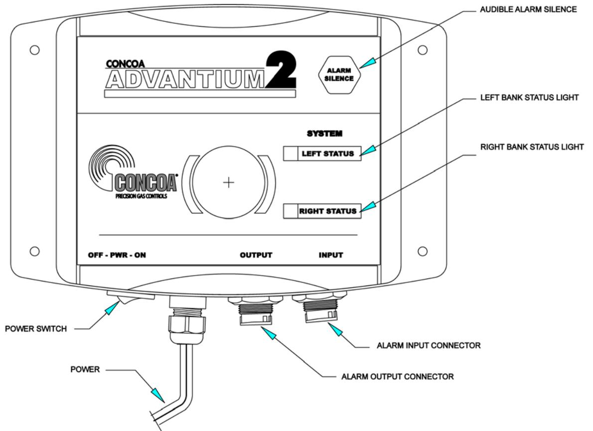
Figure 1 shows the location of the various inputs, outputs and indicators for the alarm. The Advantium 2 Plus has a universal power supply.
