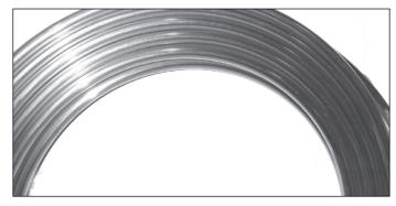
CONCOA's zero permeation 316L ¼" stainless steel seamless tubing meets the laser industry's hydrocarbon free specification. The resonator grade tubing goes a step further by eliminating all halocarbons as a result of the cold finished bright annealed processing. The cold drawn process produces a seamless surface finish that eliminates leak paths (flat spots) associated with welded tubing. The high surface finish reduces surface tension thereby preventing particulate adhesion and off-gassing.
