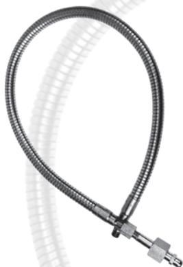
With an inner core and end fittings of 316L stainless steel, this metal hose provides an all-welded, zero permeation and flexible alternative to pipe and tubing in laser purity gas applications, even at cryogenic temperatures. The metal-lined hose is reinforced with two layers of type 321 stainless steel braid to provide maximum protection and flexibility.
