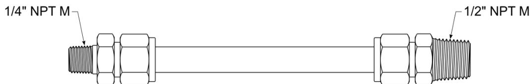
Figure 7 - Manifold Connector for the Maniflex System
