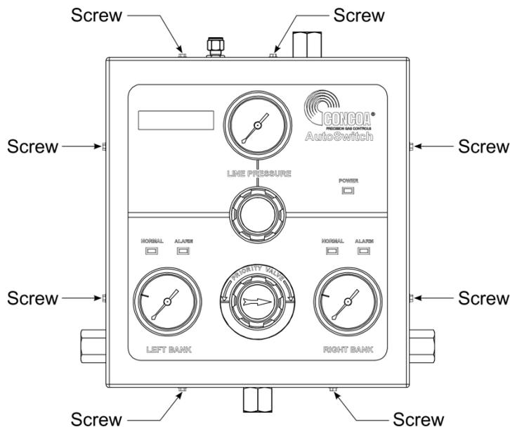
6. Slowly turn the line regulator knob clockwise. This will increase the pressure of the line. Adjust to the desired working pressure, and again check for leaks using the methods described above.
