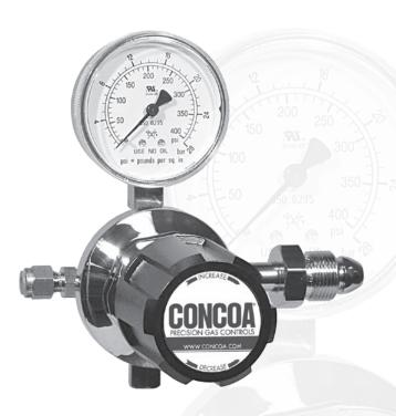
The 5260 Series regulators are designed specifically for primary pressure control of assist gases supplied from cryogenic liquid cylinders for use in medium flow up to 1500 SCFH (708 lpm) and medium pressure flow up to 200 PSIG (14 BAR) applications. The line version can be used in piping systems for lasing.
