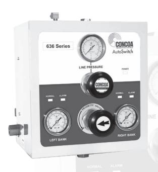
The 636 Series AutoSwitch provides a continuous supply of nonflammable industrial gases at a constant delivery pressure from two high pressure banks. Standard pressure switches enable visual alarms and an optional remote alarm to notify the user of the need to replenish a depleted bank.
