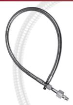
With an inner core and end fittings of 316L stainless steel, this metal hose provides an all-welded, zero permeation and flexible alternative to pipe and tubing in laser purity gas applications, even at cryogenic temperatures. The metal-lined hose is reinforced with two layers of type 321 stainless steel braid to provide maximum protection and flexibility.
