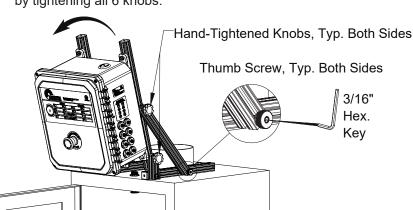
Attach the bracket to the cabinet (or any item with the correct hole pattern - see "Hole Pattern and Recommended Hole Size") as shown
