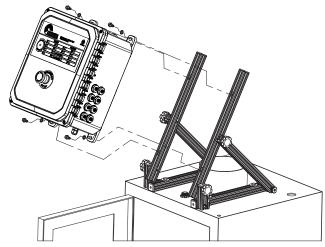
Loosen the 4 hand-tightened knobs (2 on each side of the bracket). DO NOT UNSCREW THE KNOBS COMPLETELY -
