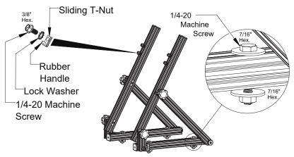
With the bracket arms tilted rearward, attach the ESO box to the bracket arms as shown below:
