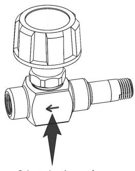
Orientation Arrow shows flow direction. Note: Valve will operate correctly in reverse direction if necessary
