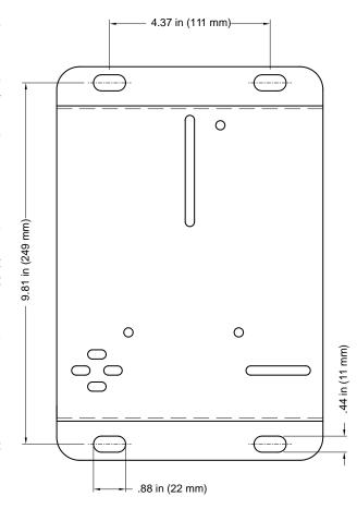
Figure 3 - Installation Bracket
