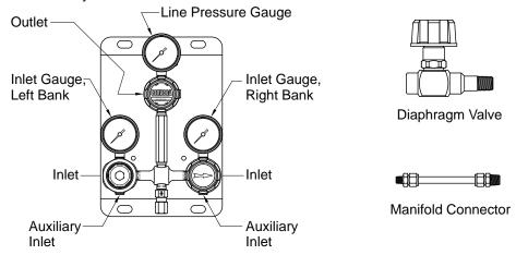
Figure 5. System Configuration for Installing the Inlet Connection
