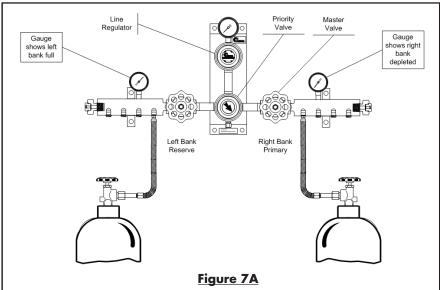
7. Rotate the 632 priority valve away from the depleted cylinder bank if both banks are high-pressure cylinders as illustrated in Figure 7B.
