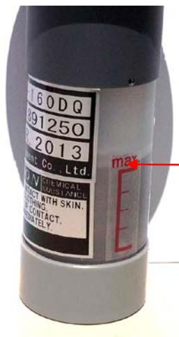
12. Turn the cell to the proper monitoring direction, (Box Nut is facing down) and confirm that the level of electrolyte is at the MAX mark. It is OK if the level is slightly above or below the MAX mark.
