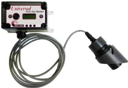
**Universal Gas Detector with remote cable connected to a duct (Max cable length 30 feet)**
