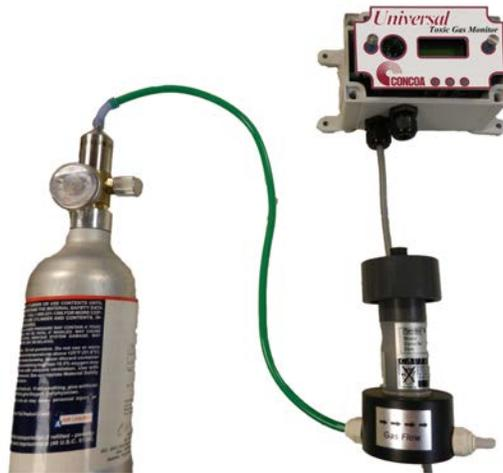
4. Push the joystick Right to enter the sensor span mode.
