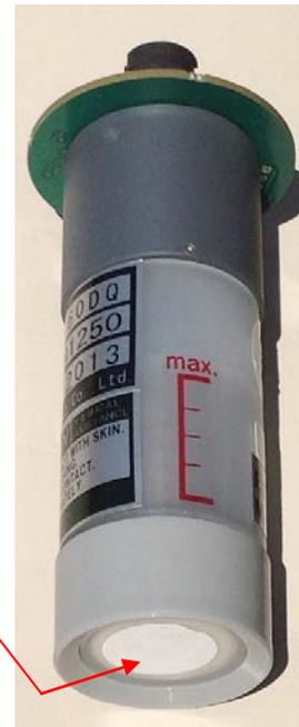
1. Place the sensor over the beaker as shown and pour the old electrolyte into the beaker.
