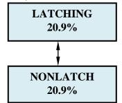
After entering the relay state the display will default back to the **Set Latching** menu. The display will scroll the following:
