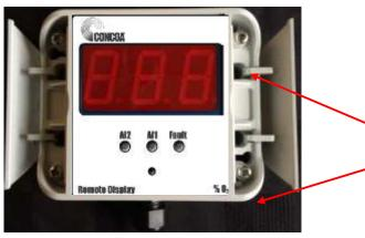
1) Open the two side doors to expose the front panel screws.
