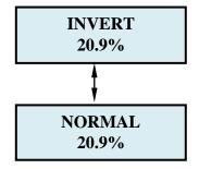
After entering the relay state the display will default back to the **Set Audio Alarm Polarity** menu. The display will scroll the following:
