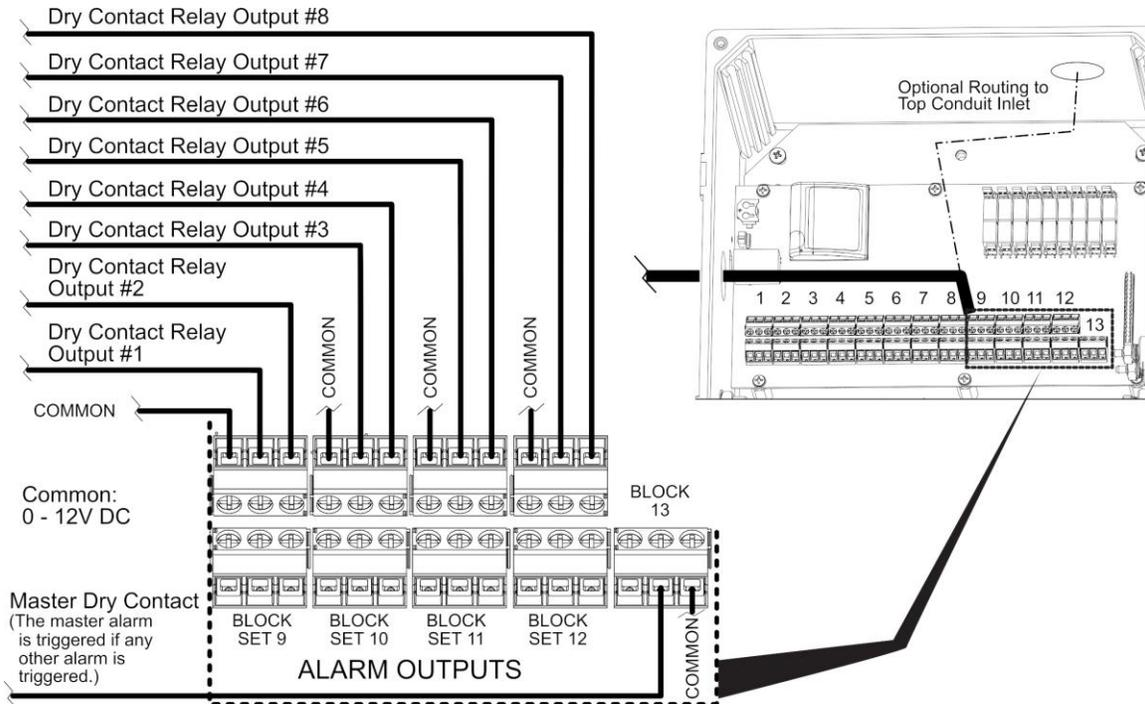
**\* STANDARD DRY CONTACT RELAY OUTPUTS SETUP**
