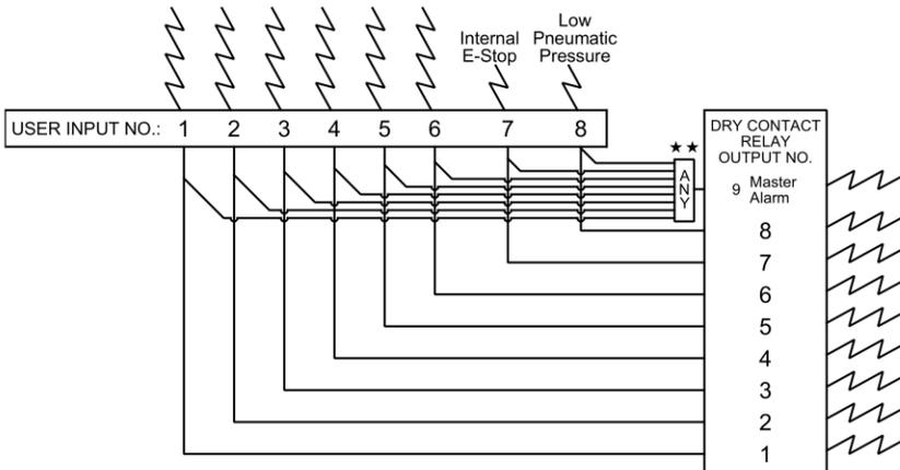
\* Except for the master alarm, all connections for both the pneumatic outputs and for the dry contact relay outputs are fully configurable via the web interface software. This includes the ability to link multiple inputs to a single output and the ability to link a single input to multiple outputs. There is no requirement for the output number to match the input number.
