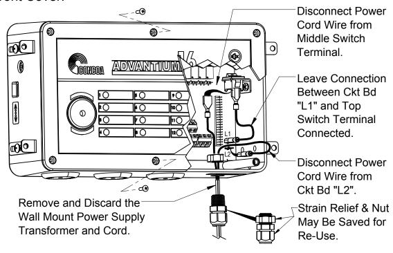
3 Supply Power and Alarm Inputs Through Holes in Bottom of Alarm Enclosure as Indicated Below:
