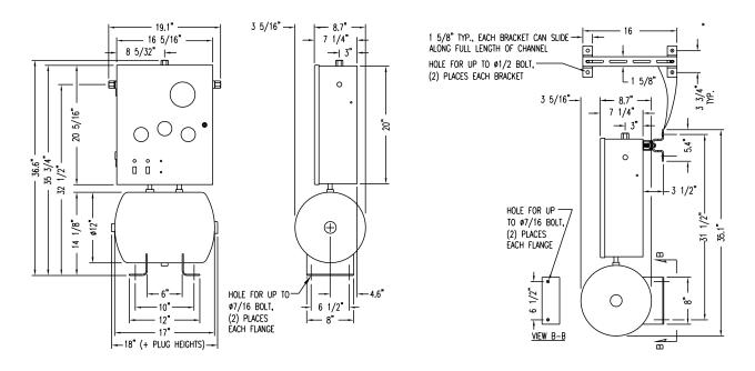
Figure 2 - Dimensions for the 655 Series BlendMaster $^{\text{TM}}$
