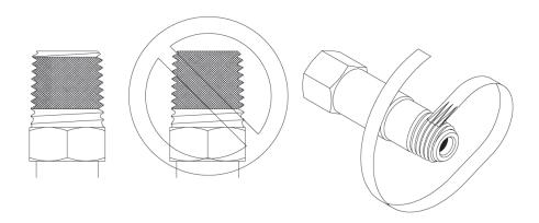
Figure 3 - Teflon Tape Placement
