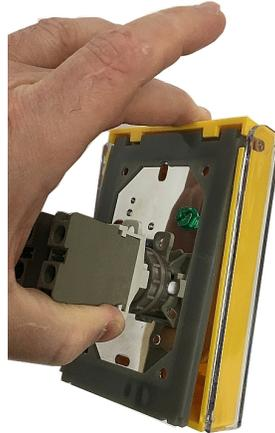
5 Connect one device to either the "Normally Open" or "Normally Closed" terminal block.
