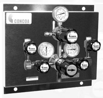
The 619 Series is an automatic pressure differential switchover that delivers a continuous supply of resonator gas without compromising purity. Low internal volume coupled with an optional inlet micro-purge virtually eliminates gas contamination. In addition, the stainless steel diaphragms and double seal relief valve enable the 619 to achieve 1 x 10-8 He scc/sec leak integrity.
