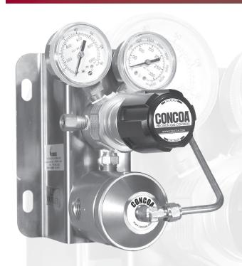
The 623 Series is an ultra high flow gas delivery system for laser assist gases. Typically these gases are supplied from low pressure (less than 600 PSIG/42 BAR) cryogenic supply systems. The 623 is designed for direct installation to the external vaporizer. The dome-loaded, balanced stem seat design allows for full flow capacity that may be required for the assist or process gases, and ensures constant delivery flow and pressure regardless of supply source inlet pressure fluctuations.
