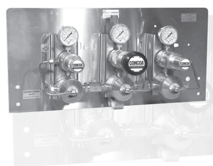
The 639 Series Assist Gas Switchover is a primary-reserve system designed to provide a continuous supply of laser assist gas from two high pressure sources. The system comes pre-mounted on a stainless steel panel, complete with flexible hoses for connections to bulk high pressure sources.
