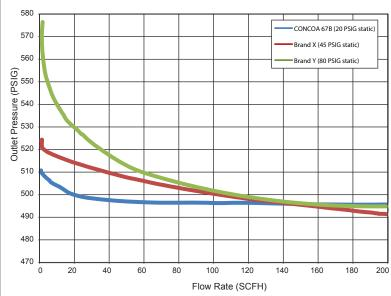
Compared to traditional ½" dome-loaded regulators, the 67B series regulator provides industry leading low static increment, increasing the precision and response time of pressure control.
