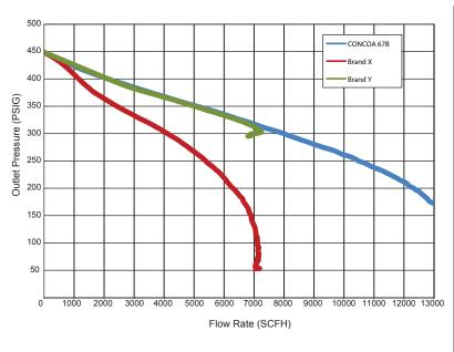
The 67B Series regulator provides significantly larger flow capacity then traditional  $\frac{1}{2}$ " dome-loaded regulators.
